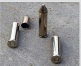
Calibre .357 Magnum Bullet weight 10.2 g Impact at 430 m/s Impact force of coned bullet 943 J
